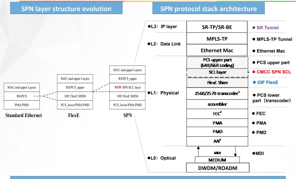
SPN innovatively introduces SPN channel layer, integrates TDM and packet switching, and integrates L0 layer to L3 layer into a whole.
