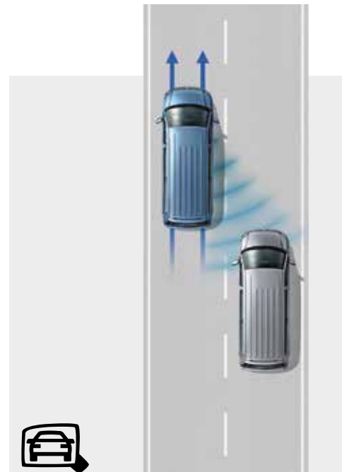
Lane Change Assist "Side Assist". Displays a warning signal in the door mirror if one of the system's sensors registers a vehicle in the blind spot when changing lanes. Available on Short Wheelbase Van and Crewvan only.
