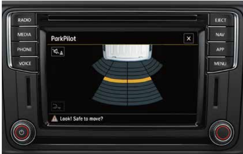
Rear Park Distance Control. Emits audible warnings when obstacles are detected behind the vehicle when parking, and also provides a visual display of the vehicle's distance from the obstacles (Discover Media shown).
