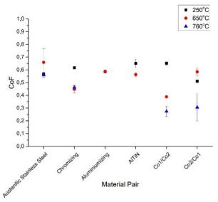
Figure 7. Friction performance of concepts at the tested temperatures.
