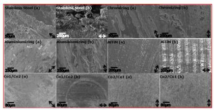
Figure 11. InLens SEM images of the wear scars of the pins (a) and plates (b) subjected to tribology testing at 250°C. Arrows indicate the direction of sliding.
