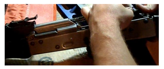
Then insert your dust cover, front first into the notch in the front trunnion and hook the back of the spring assembly into the square hole ...
