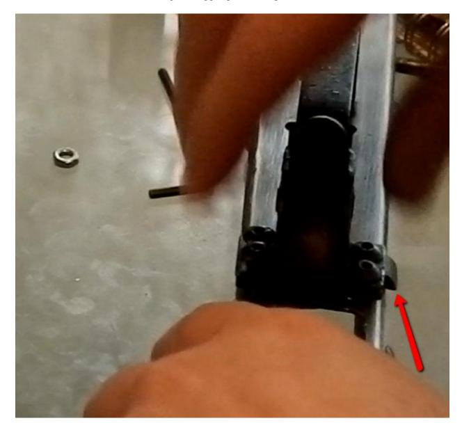
Notice the safety selector catch is on the right hand side of the receiver (that's that little notch with the arrow pointing to it.
