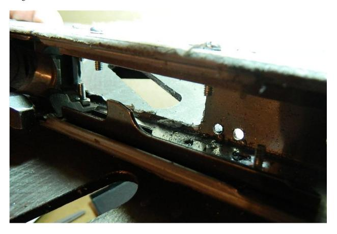
You'll also need to redrill through the center support hole you already drilled because that center support will go through the rail as well. In this pic, you can see on the right side rail that the center support and hammer holes are redrilled through the lower rail again:
