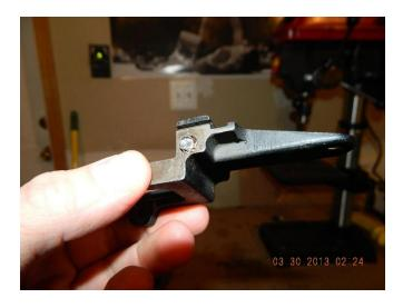
Start with the smallest bit you can get, clamp down and drill through the rivet all the way through first. Here you can see the hole I drilled all the way through:
