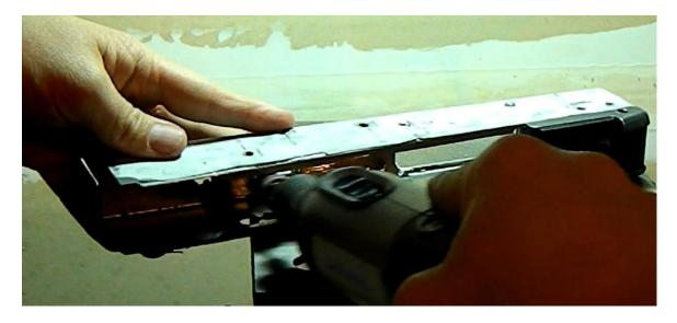
Then just keep test fitting after each go around with the dremel to see if it moves freely. when you can slide the bolt carrier on the rails all the way to the front of the receiver where it butts into the front trunnion with no binding then you know that you've trimmed them enough:
