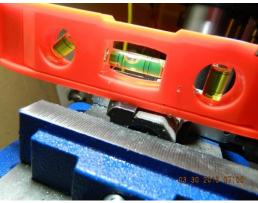
And then just start drilling all 4-6 holes you need to drill. Now these holes are all going to take a 10-32 thread -- for your screws to hold it together (from your screw kit). Unfortunately, that correlates to a #21 drill bit -- which I didn't have -- so I went the next size DOWN to 5/32 size drill bit for these 4 holes in the trunnion. Again, always start with the smallest size drill bit you're comfortable with -- and then "step drill" up to the final size (5/32):
