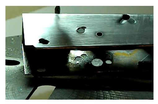
Next, make sure you tap the rear trunnion holes for the 10-32 threading for your screws:
