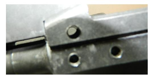
Set it up in your vice, check your levels on the x and y axis (very important) and try to drill all the way through all in one shot. Be VERY careful because the trunnion metal is MUCH softer than the barrel and you don't want to let the bit walk and mess up your trunnion by "egging" out one side.
