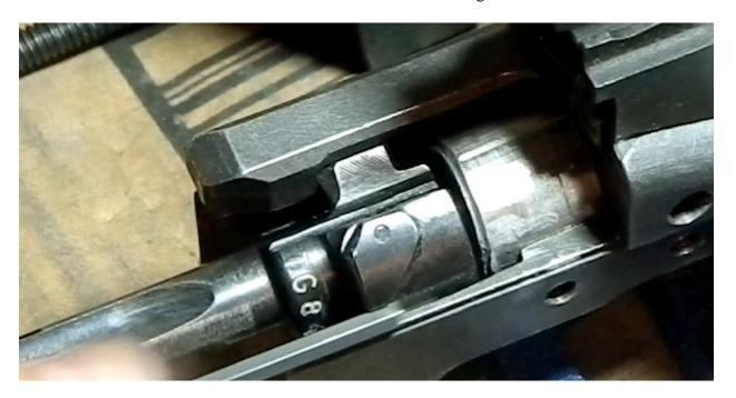
Now, to get to this point, we had to do a little adjusting. So you'll have to move the barrel in or out of your trunnion just a LITTLE BIT AT A TIME because it is always a small difference that can make it fit or not fit.
