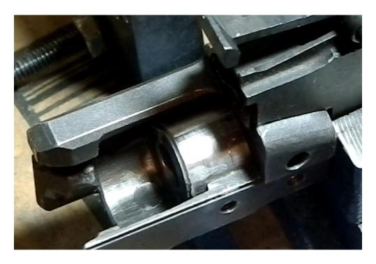
As shown in the picture below, you should at least have enough width between the ridges in the front trunnion and the barrel to fit the bolt, for it to spin:
