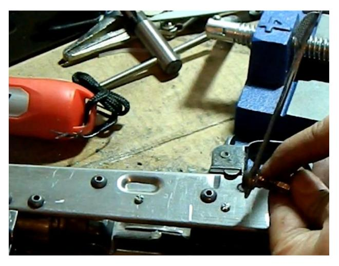
And I also had to notch the part where it would clear the disconnector part of the trigger assembly:
