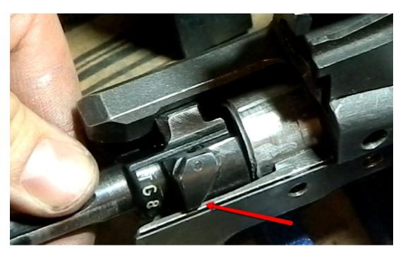
Now, the "Go Gauge" was a success, let's now make sure that the "no go guage" is a failure! In this case, the no go gauge should NOT be able to turn completely to the right and rest on the front trunnion. Here is the no - go gauge:
