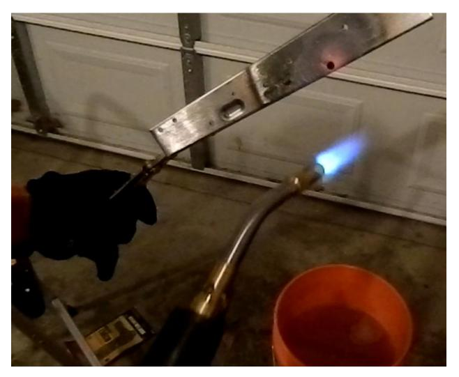
Do that will both sides hammer and trigger hole. Then wait a little for it to cool off, and scrape off the extra carbon buildup as best you can for
