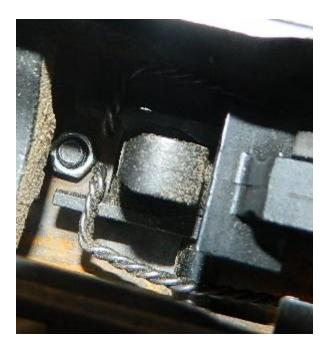
The last step, my safety selector was a bit of a pain! I had to do a lot of trimming and grinding to get it to fit. In my case I had to widen the part where it would go in the hole, so that it would fit my receiver:
