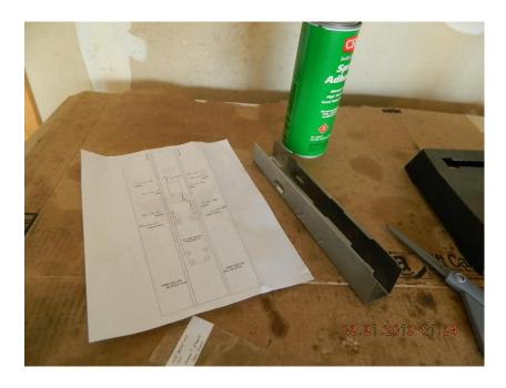
Using spray adhesive and a lot of patience, cut it out and paste it on (if you are using a 80% blank like I was then make sure your magazine holes and pistol grip holes and trigger holes are all matching in the right spots on the template -- that will make it easier! Here it is done:
