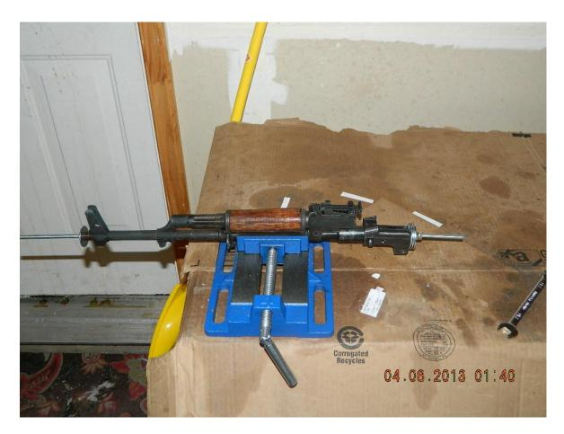
That was a total disaster -- the all-thread broke (remember it was the home depot zinc plated stainless steel junk) and the washers all bent probably driving my front trunnion on crooked.
