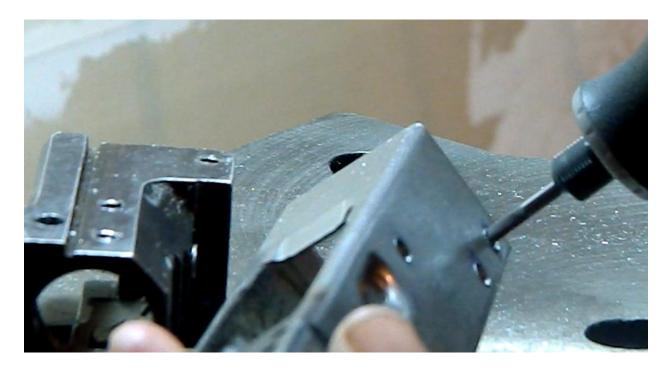
Just get your receiver holes to line up to the trunnion holes, and tap the trunnion holes and you'll be fine. (picture below is me tapping the receiver but just tap the trunnions -- and make sure it's not crooked like this)
