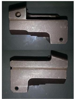
Front trunnion only has one of the six holes drilled for the "rivets". Also the barrel pin hole is not drilled all the way through. So I'll have to do that.
