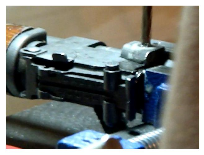
I ended up getting a center cutting carbide endmill in 7/32" from Amazon.com for this: http://www.amazon.com/gp/product/B003CYKFHO/ref=oh\_details\_o05\_s00\_i00?ie=UTF8&ps c=1 -- it cut through pretty easy, but I did damage a few of the "flutes" and also I did end up egging out the other side of my barrel hole because I didn't have it as square as possible!
