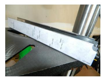
Step 5: Drilling the receiver holes using the template
