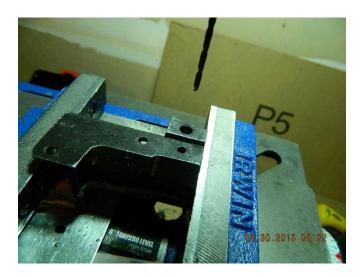
Now you need to drill the barrel hole (unless yours is already drilled) mine wasn't so I had to drill out the barrel hole as best I could--for sizing this hole, there was already a "pilot" hole for the barrel hole that was there -- but it wasn't drilled all the way through (as you can see in the picture below):
