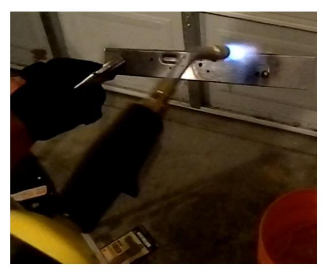
Don't go all the way to red hot this time, just to blue-ish color then let it air cool (no quenching!). Now, when I did this I did it back to back. It would be SMARTER to take it and clean it as best you can after the first heating and quenching so that you can better see if the steel is turning colors.
