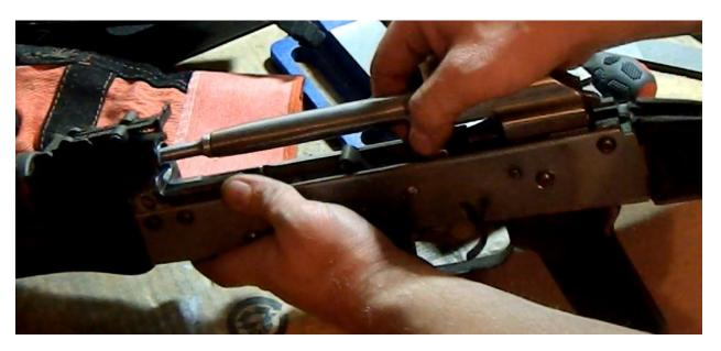
Then stick in the big spring into the bolt carrier and find where the other end connects to the rear trunnion ...
