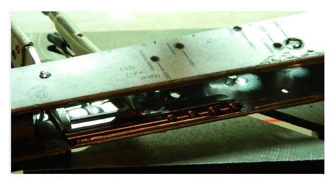
The size drill bit that worked for me was the 1/4" drill bit, but that is just a starting point! You are looking for a drill bit that allows you to line up the "ledge" of the front trunnion with the top of the rail, as shown in the highlights by the red line below:
