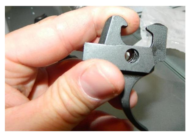
Your're going to take the spring and put it on the hammer first, and crank it up and then use the zip tie to hold the spring to the hammer to make it easier to install:
