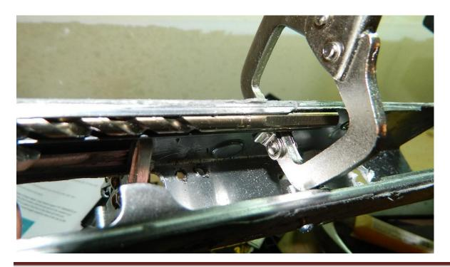
Again, you'll want to fit it with a drill bit, and it does NOT matter if you use the same size drill bits on both sides! what DOES matter is that, again, your rail is in line with the front trunnion -- they need to be level!
