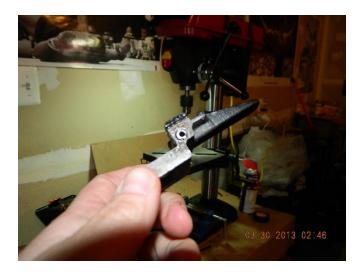
Then, you can work your way up in bit sizes -- step drilling -- until you remove enough of the material that you can just grab a punch and bang out the remaining parts of the rivet. Here's what it looks like once you've punched the rivet out:
