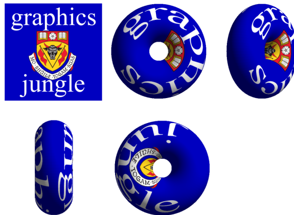
Figure 3.1: Top Left: A 2D texture. The rest of the figure shows a torus from various angles. It has been texture mapped according to Equation 3.1.
