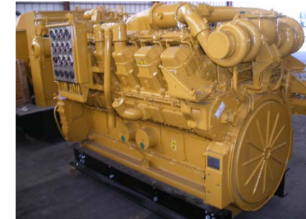
2250 bhp Diesel Engine: 15,000lbs
