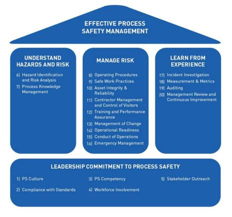
Figure 4: Twenty elements for effective process safety as adopted by Unilever
