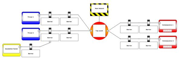
Figure 2: Typical Bowtie Diagram
