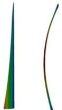
Finite Element modelling assists in identifying the deformed shapes of the multi-stable states.
