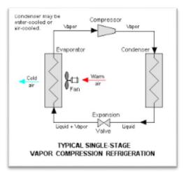
from the air inside the refrigerator box to the ambient air outside of the box.
