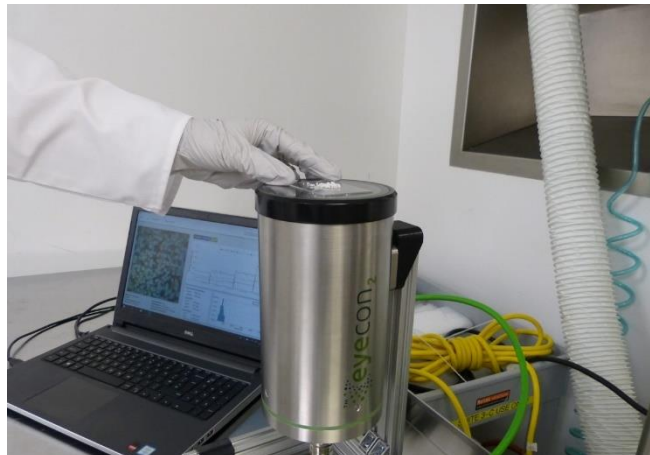
Image 5: Real-Time At-Line Configuration of Eyecon 2 for CPS Analysis
