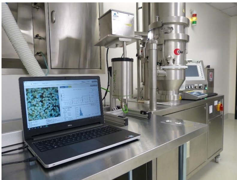
Image 3: Eyecon 2 installation next to a Glatt CPS Processor with Pelletization Sample Interface
