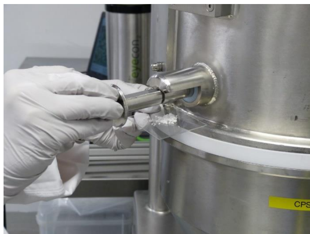
Image 4: Samples taken directly to Microscope Slides for immediate measurement
