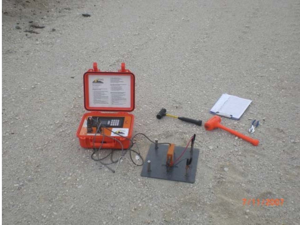
Figure 13 - Electrical Density Gauge (EDG) Setup
