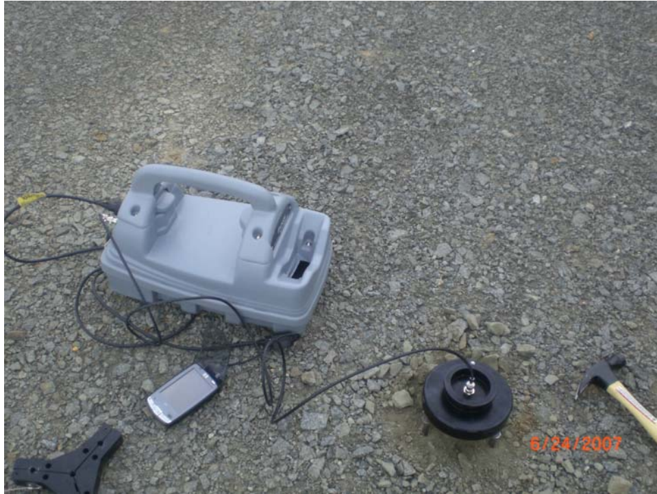
Figure 12 - Moisture Density Indicator-MDI 2000 (TDR) Setup
