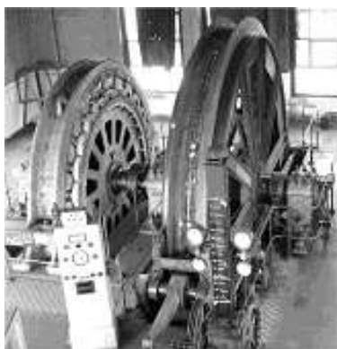
Fig. 4. DEMAG winding engine
