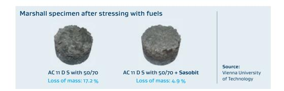
Pure **Sasobit** is nearly insoluble in fuels. **Sasobit**-modified asphalt mixes are therefore much more fuel-resistant. Fuel resistance is enhanced even more because **Sasobit** allows for an optimal compaction.
