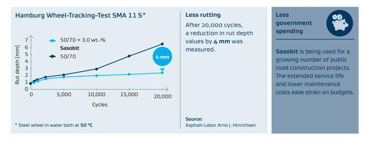
**Sasobit** has also yielded outstanding results – mostly as co-modification of PmB – when using it for heavy-duty asphalt pavements. Such asphalt mixes are used for areas under high dynamic and static loads.
