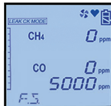
Leak Check Mode
