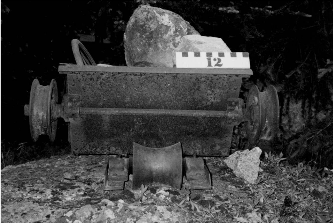
Figure 4-34. End view of the Lawson-style ore car. The cable guide wheel in the foreground is not part of the car.
