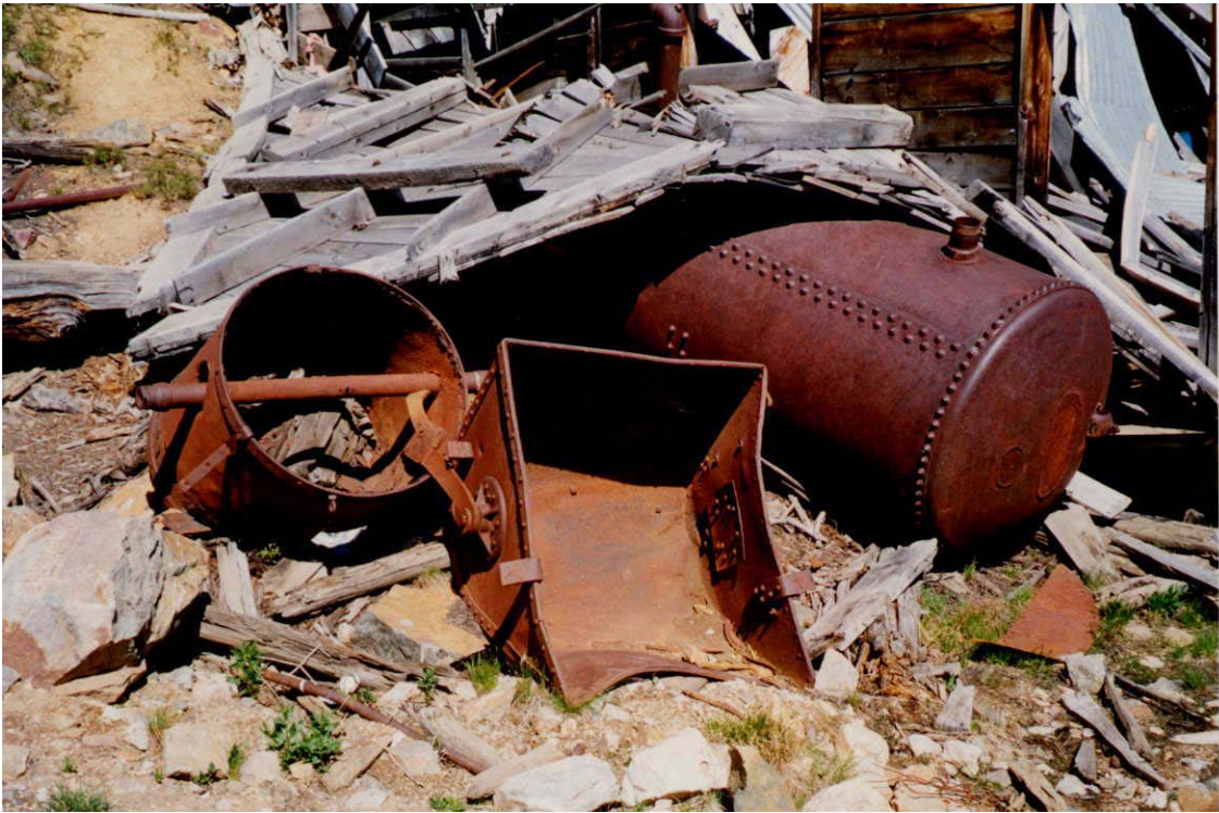
Figure 4-25. Another ore car (center) next to a compressor tank (right) and an unidentified “homemade” bucket device (left), near the discharge terminal.
