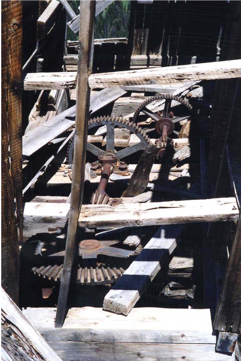
Figure 4-21. Detail of gear reduction system.
