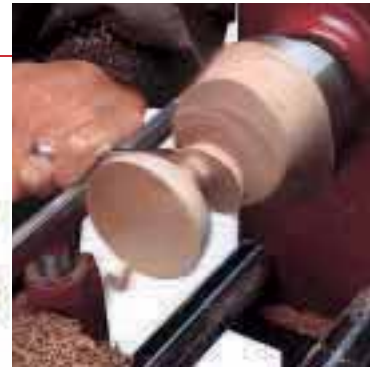
Turning a goblet with off-set stem using 0, 10 and 20mm settings.
