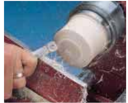
External shaping (Ref:827H)
