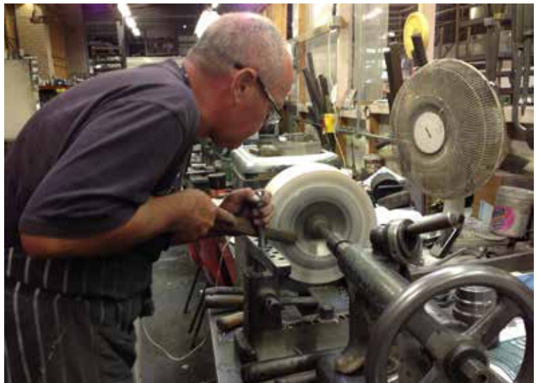
Brian Swift spinning one of Gordons' designs at A.R. Wentworths factory in Sheffield.
