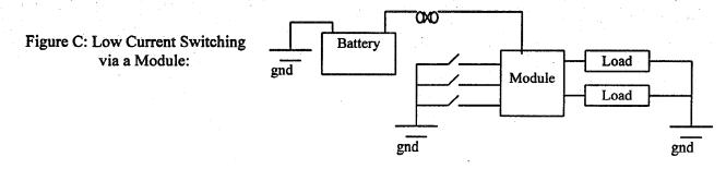
The addition of a multiplexed link between these modules allows information to be shared whilst REDUCING the number of harness wires required (see figure F, later in paper). Once a switch or load is wired to one module, the status or control of that wire is available to all the other modules on the network via the multiplexed link.
