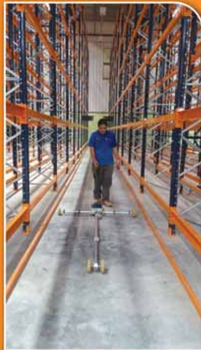
SUPERFLAT FLOOR SURVEY
