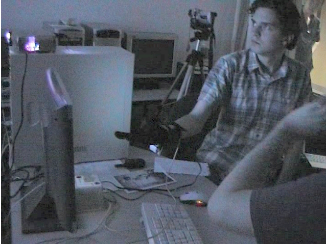
Figure 10 - Bee Actor controlling the virtual flock with a motion tracker and data glove
