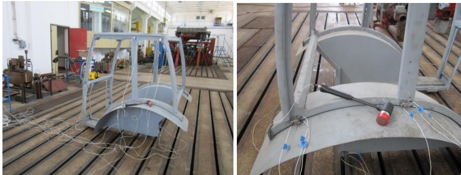
Fig.4. Assembly for conducting the modal analysis experiments of the tractor cab. Detail on positioning the accelerometers for measuring the vibrational response
