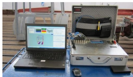
Fig.7 Data acquisition equipment, during a measurement sequence under SDTC
