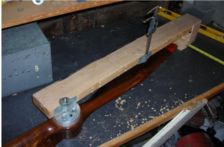
Figure 4: The apparatus used to find the propeller geometry
