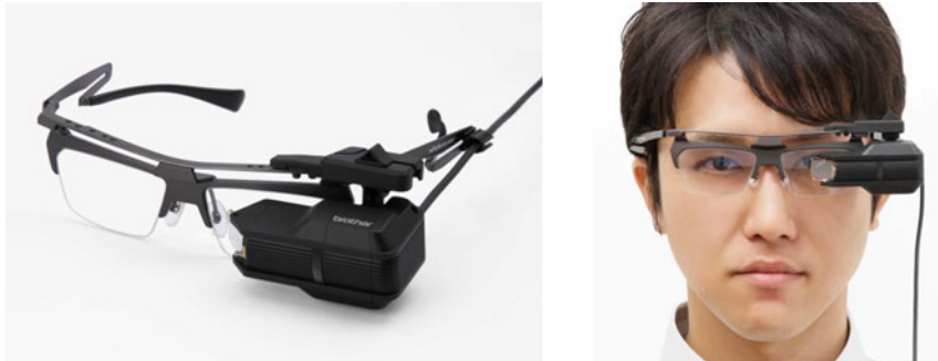
Figure 95. A commercially available see-through head-mounted display 'AiR-Scouter' by Brother Industries Ltd. (Images courtesy of Brother Industries).
