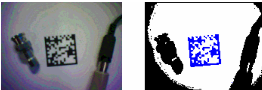
Figure 29. The left image shows how the image gets darker radial from the centre due to the camera's poor characteristics (vignetting). The right image shows how this affects the threshold. The detected marker is blue and the rest of the threshold areas are black. (Image: VTT Augmented Reality team).
