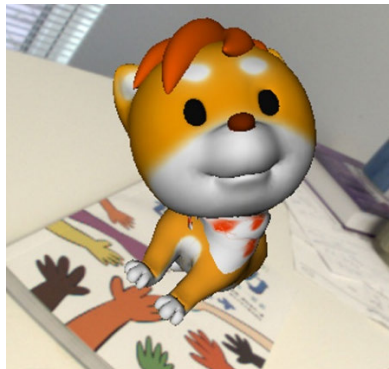
Figure 51. Example of natural image detection: An animated character is augmented on the top of a book. The detection is based on features in the cover image. (Image: VTT Augmented Reality team).
