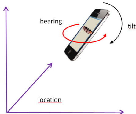
Figure 62. Different sensors define different properties of the object's pose. For example, GPS indicates the object's location, an accelerometer and magnetometer give the tilt (of all three axes) and a compass gives the object's bearing. All these together are enough to define the object's (6 DOF) pose.
