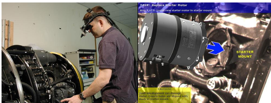
Figure 11. ARMAR: augmented reality for maintenance and repair (image courtesy of Steven Feiner).
