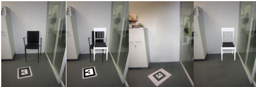
Figure 69. Example of diminished reality, images from left to right: original image, augmentation over existing object, diminished image, augmentation over diminished image.
