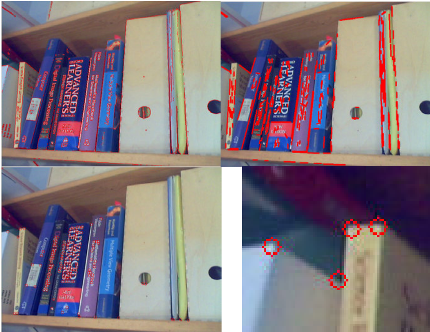
Figure 61. Examples of detected edges (upper left), lines (upper right), and Harris corners (bottom left) are marked with red. At the bottom right is a zoomed part of the image with the detected corners.
