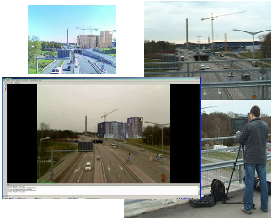
Figure 9. Outdoor visualisation: the user (bottom-right) sees the actual environment (top-right) and the augmented reality with the new building project through the display (bottom-left). The augmentation is adapted to the environment lighting (top-left). (Image: VTT Augmented Reality team).
