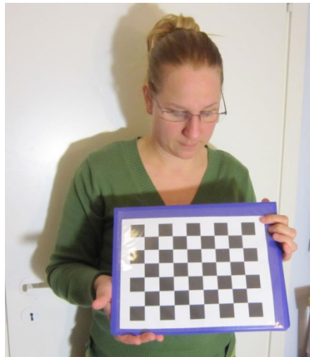
Figure 115. Example of a planar calibration rig with a chequerboard pattern.
