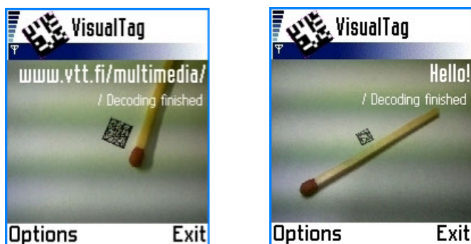
Figure 57. Screenshots of our marker detection system [11]. With the add-on lens, it is able to recognise tags with a cell size of only 0.06 \text{ mm}^2 . The marker in the left image contains the URL “www.vtt.fi/multimedia” and the marker in the right contains the word “Hello!”
