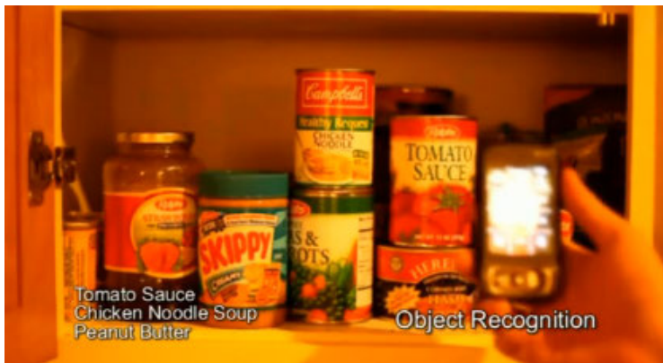
Figure 20. The LookTel smartphone application for the visually impaired recognises objects and characters, and reads aloud things at which the user points using the mobile phone (image courtesy of LookTel).
