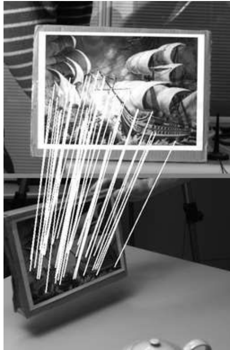
Figure 52. Feature matching with BazAR (Image courtesy of Vincent Lepetit).
