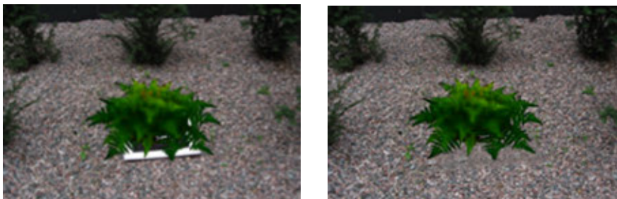
Figure 78. Visible marker is distracting, even if it is only partly visible under the augmentation (on the left), whereas the hidden area blends nicely with the rest of the image (on the right).
