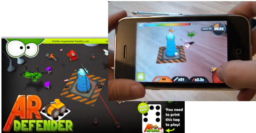
Figure 13. Mobile augmented reality game AR Defender uses markers for pose tracking (Images courtesy of Int13).
