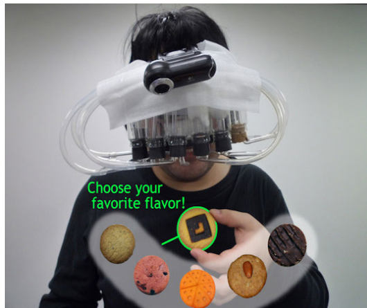
Figure 22. Meta Cookie setup: instead of neutral tasting sugar cookies, users see augmented cookies and are given corresponding smells image form [62].
