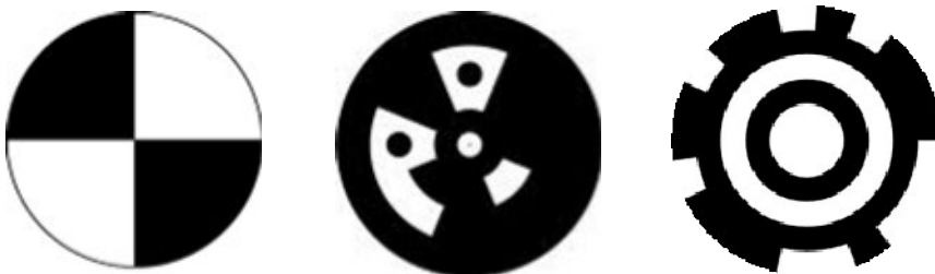
Figure 49. On the left, an example of a simple position marker used in photogrammetry; in the middle, a circular marker used by InterSense [109] and on the right, SpotCode [110].
