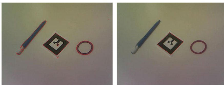
Figure 25. An example of edge detection using ALVAR. On the left: the edge contours detected on the threshold image (Figure 24) are superimposed onto the original image with red. On the right: the remaining edges after applying the four-corner test and size test.
