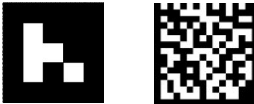
Figure 46. On the left, a simple binary marker (ID marker), and on the right, a binary data marker. The binary marker on the right is an example of our marker system presented in [11].
