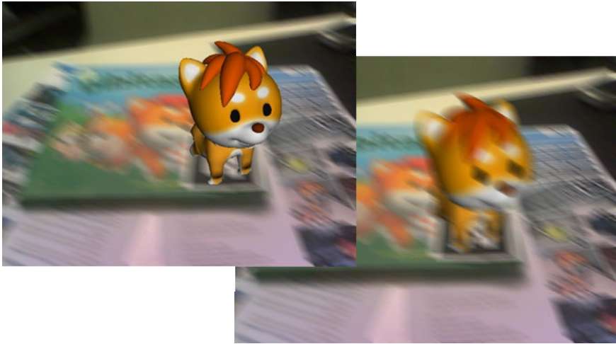
Figure 68. An example of motion blur adaptation: on the left augmentation without blur adaptation, on the right with adaptation.
