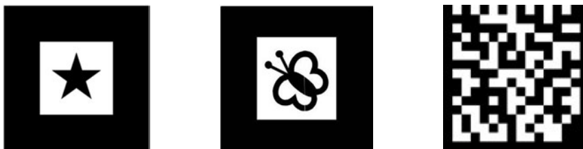
Figure 28. The marker on the left has exactly one hole (a white area) and the marker in the middle has three holes. The marker on right is an example of a binary marker with numerous strong edges. A system can use this kind of knowledge for fast acceptance/rejection tests.
