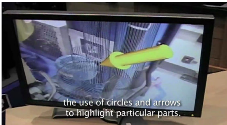
Figure 64. In visualizing a maintenance task, NPR rendering is appropriate: the highlighted arrow draws the maintenance worker's attention to a particular part (image from [15]).
