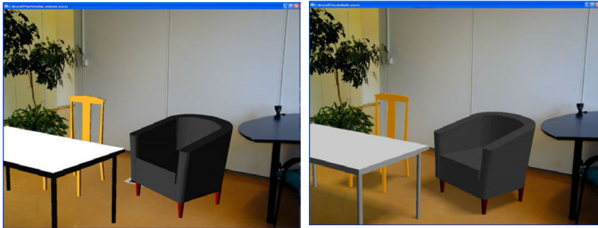
Figure 65. Example of realistic virtual lights and shadows from our interior design application [12]. On the right, the user has manually adjusted the virtual light sources based on real ones and the soft shadows of the virtual objects are similar to real shadows. We have also removed the marker from the resulting image for a better visual appearance.
