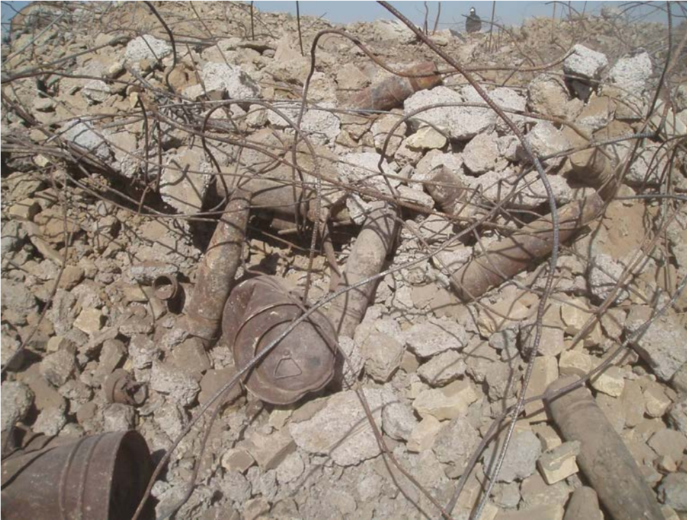
Figure 10.7 “Blow-and-go” tactics often resulted in ordnance buried beneath tons of concrete rubble and steel rebar.
