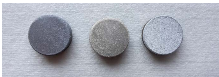
Figure 19: Three of the coatings used for optical measurements; from the left: APS YSZ + Cr, APS YSZ + Ag, and PS-PVD YSZ.
