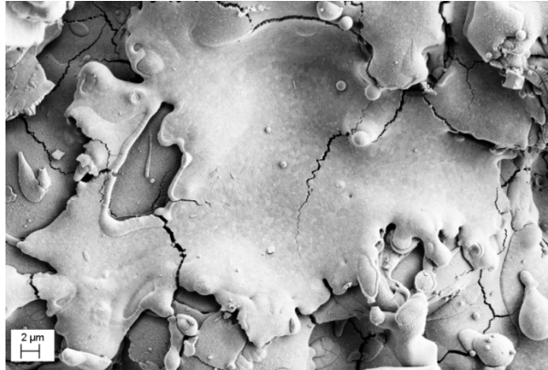
Figure 4: The surface of an APS YSZ coating, showing how a molten particle has flattened on impact.
