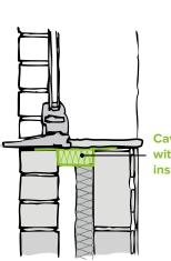
**Cavity closer** with a PU/PIR insulation core
