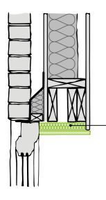
Use a thermal laminate plasterboard reveal/soffit
