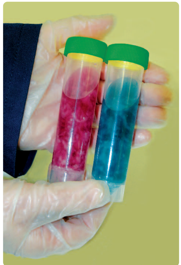
AES v RCF solubility test kit : clearly identifies the fibre already installed.
