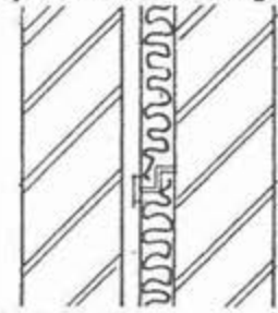
Fig.1.28 Recommended cavity-insulation with a rigid board
