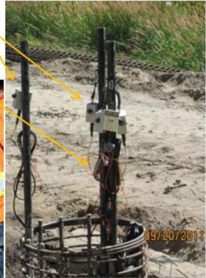
Method B - Uses Embedded wires attached to reinforcement cage
