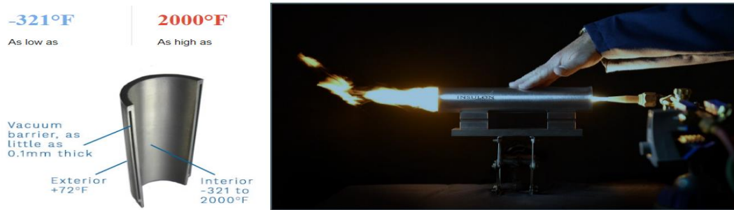
Figure 2 Insulon® performance (ref. 2)
