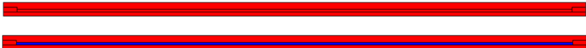
Figure 3 Model setup - top: solid tube; bottom: air gap within the tube thickness
