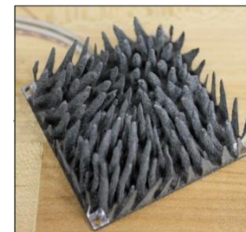
AlSi12 Rapid Prototype
