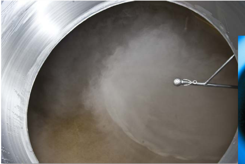
Heating up the mash and hold the temperature break
