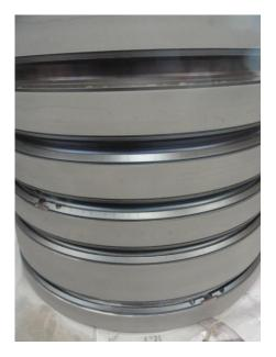
Spool with Al2O3 Machine Element Clearance Control coating.
