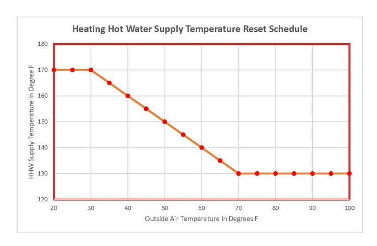
Note: HHW supply temperature range is 130 to 170  $^{\circ}$ F with reset based on outside air temperature. Actual loop temperature may vary +/- 5  $^{\circ}$ F from target.
