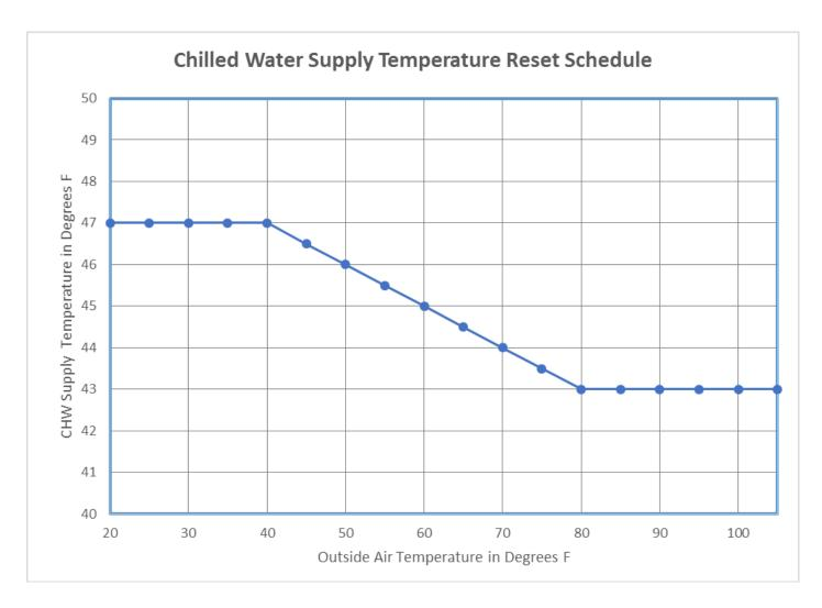
Note: CHW supply temperature range is 43 to 47  $^{\circ}$ F with reset based on outside air temperature. Actual loop temperature may vary +/- 1  $^{\circ}$ F from target.
