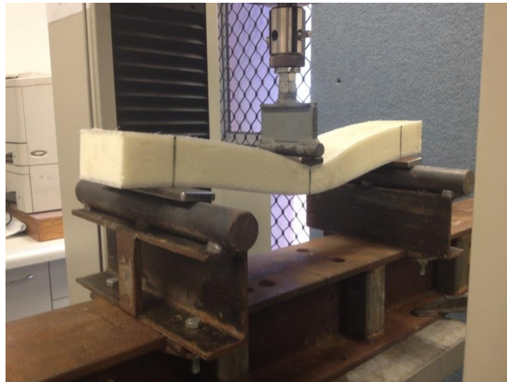
Figure 32 - Core crushing failure mode
