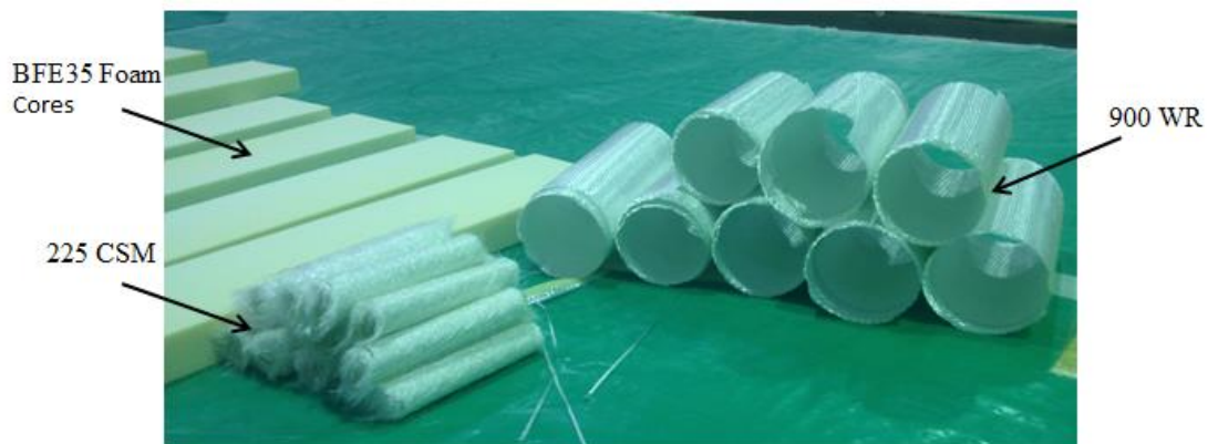
Figure 23 - Foam core, chopped strand mat and woven roving glass
