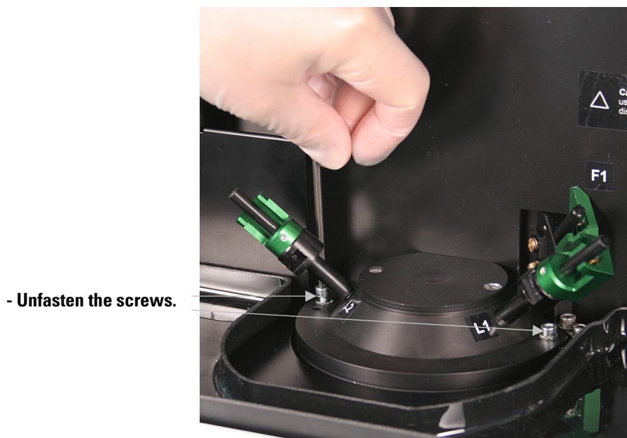
Figure 3–38. Removing the dispensing base
