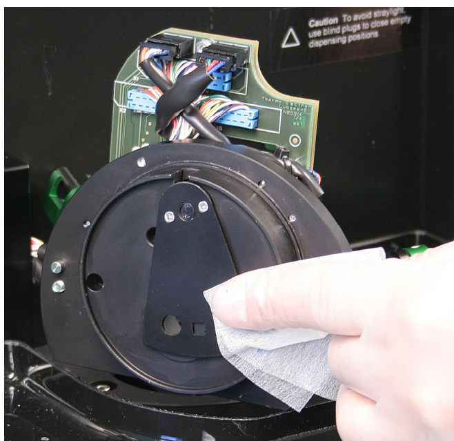
Figure 5–57. Cleaning the Varioskan LumiSens base from the bottom
