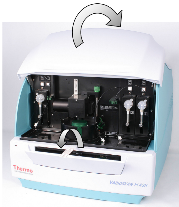
Figure 3–24. Dispenser sliding cover and measurement chamber door opened
