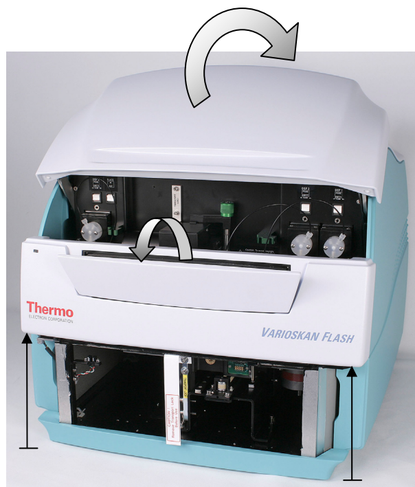
Figure 5-51. Front cover removed
