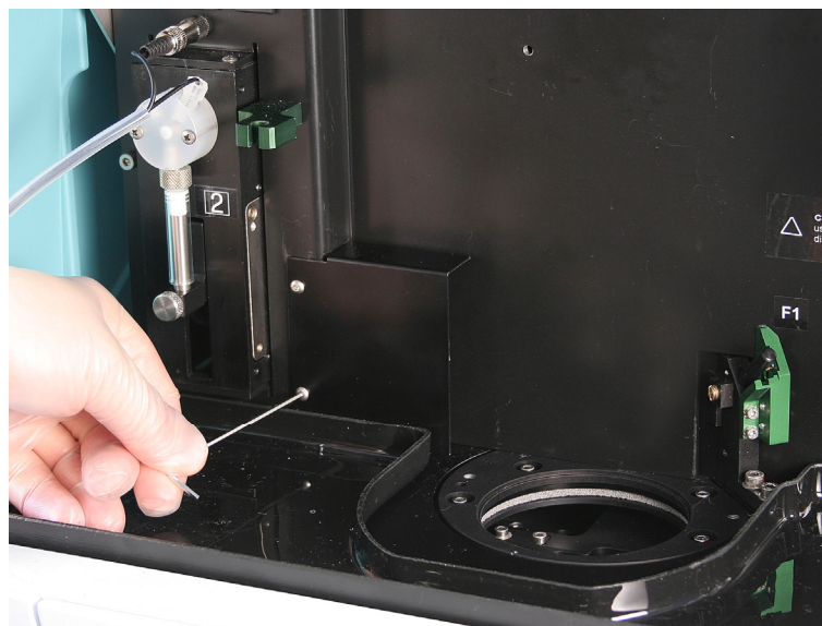
Figure 3–40. Removing the connector protection shield
