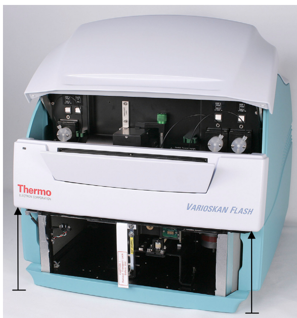
Figure 3–25. Front cover removed
