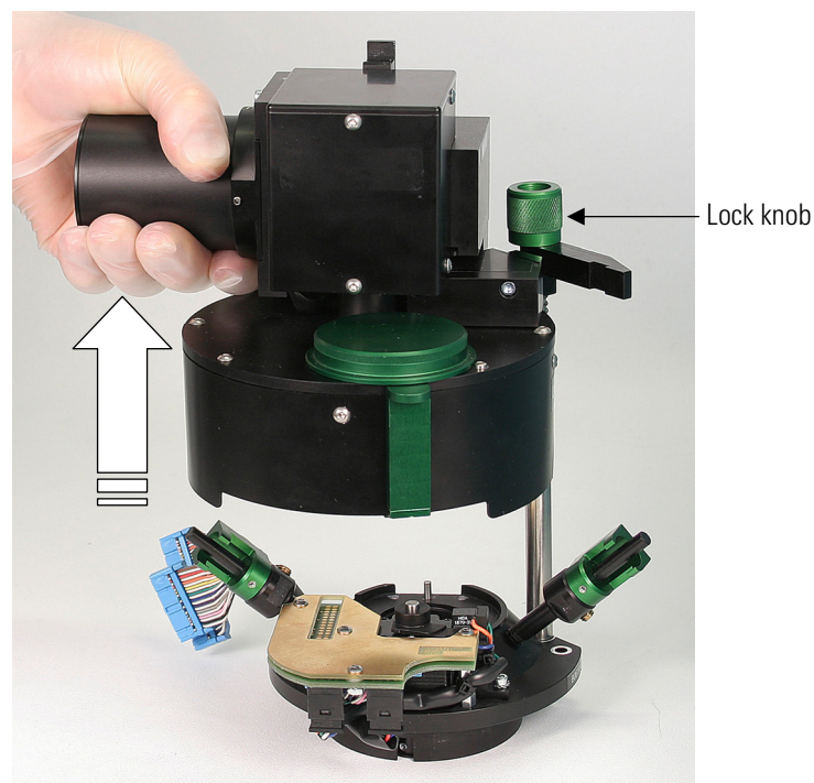
Figure 3–39. Releasing the green lock knob
