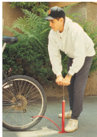
FIGURE 24.3 ▲ Do work on a pump by pressing down on the piston and the air is warmed.
