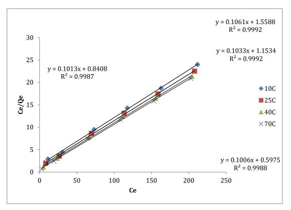
Fig 1. Langmuir adsorption isotherm for batch adsorption of  $Fe^{2+}$  at various temperatures.
