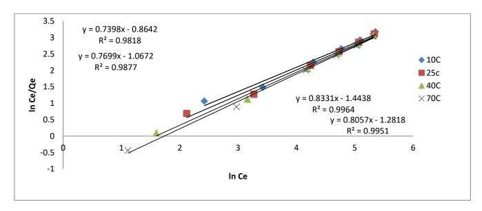
Fig 4. Redlich- Peterson adsorption isotherm for batch adsorption of Fe<sup>2+</sup> at various temperatures
