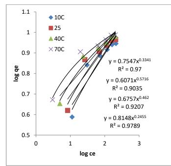
Fig 2. Freundlich adsorption isotherm for batch adsorption of  $Fe^{2+}$  at various temperatures.
