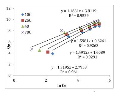
Fig 3. Temkin adsorption isotherm for batch adsorption of  $Fe^{2+}$  at various temperatures.
