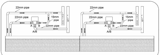
Designer vertical LPHW stacked units will be supplied with a suitable pipe connecting kit and balancing valves to ensure heat output is even over the whole height of the air curtain.
