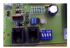
DIP switches fitted on the Ecopower board provide a selection of optional features as described above. Isolate and switch electrical power off before configuring and/or changing any DIP switch settings.
