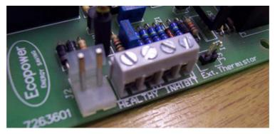
• An **INHIBIT** two screw terminal fitted on the Ecopower board for BMS remote On/Off feature.
