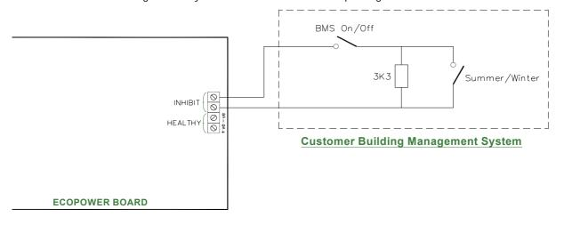
• A **HEALTHY** two screw terminal is included on the board for a fault signal indication if the electric elements overheat cut-out has operated. A healthy system provides a 24V DC signal at the terminals compared to an overheat fault which provides OV DC.
