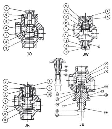
When properly applied and installed, AMOT thermostatic valves should operate for years with minimal maintenance. An inspection at two or three year intervals is adequate to detect and make provision for normal wear. The frequency of element replacement will depend on the operating conditions and the type of fluid being controlled. Because of the diaphragm and plug construction of the wax actuated element, calibration will be maintained over thousands of cycles.
