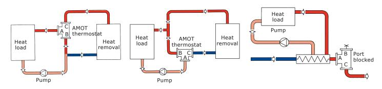
AMOT model J thermostatic valve is available in various versions to fit different applications:
