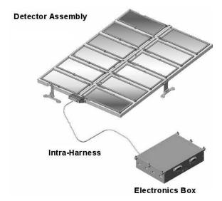
Figure 1. The Student Dust Counter provides  $\sim 0.1 \text{ m}^2$  of sensitive area. It was designed to measure the mass of IDPs in the range of  $10^{-12}$  to  $10^{-9}$  g. It continues registering the impacts of bigger dust particles without the ability to determine their mass. It weighs 1.6 kg and consumes 5.1 watts of average power.
