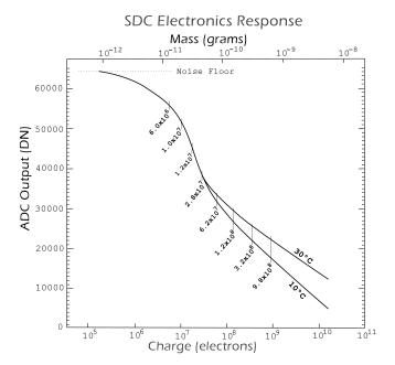
Figure 5. A typical SDC charge to DN response curve. Temperature dependent changes in gain are characterized during calibration. In-flight temperature monitoring and charge injection (the 8 onboard stimulus levels are indicated as vertical dashed lines) support post-processing correction for gain curve shifts.
