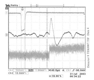
Figure 6. Example of output pulse from a PVDF sensor to a  $3.1 \times 10^{-11}$  g iron particle impacting at 4.52 km/sec. The top trace is from the accelerator charge induction tube (100 mm, 6.1V/pC), the middle trace is the output of the shaper  $(1.47 \times 10^{-5} \text{ mV/e})$  and the bottom trace is from the CSA  $(7.3 \times 10^{-7} \text{ mV/e})$  (note: gains are not flight values).
