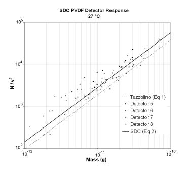
Figure 7. Dust impacts on SDC prototype PVDF sensors. Plot of ratio  $N/v^3$  vs projectile mass. N (electrons) is the measured detector signal and v (km/s) is projectile velocity reported by the dust accelerator.
