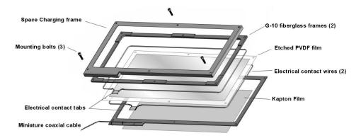
Figure 2. Exploded view of a single SDC PVDF detector. The detector is mechanically bonded with structural epoxy. Electrical connection from the PVDF metalization to the signal wires is through silver filled epoxy. The signal wires are soldered to miniature coaxial cables leading to the system electronics. Three mounting screws tie the space charging frame and the detector to the underlying honeycomb support panel.
