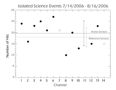
Figure 10. The number of single events registered on each of the SDC channels (with the exception of channel 11). These were recorded between 7/14/2006 and 8/15/2006, during a total operating period of about 2.5 weeks. The average number of hits and the  $\pm 1\sigma$  error bars are also indicated for both the front (continuous line) and the reference (dashed line) sensors.
