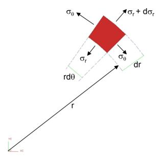
Now consider and element at radius r and defined by an angle increment d $\theta$  and a radial increment dr. By circular symmetry, the stresses  $\sigma_{\theta}$  and  $\sigma_{r}$  are functions of r only, not  $\theta$  and the shear stress on the element must be zero. For an element of unit thickness, radial force equilibrium gives:
