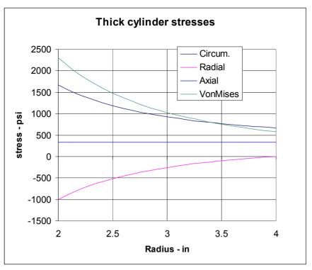
Example of cylinder with  $P_i = 1000 \text{ psi}$ ,  $r_i = 2^{\circ}$  and  $r_o = 4^{\circ}$
