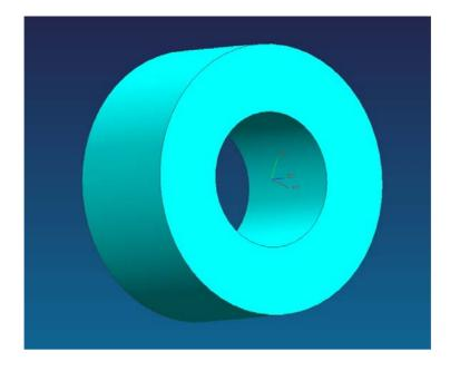
Consider a thick walled cylinder with open ends as shown above. It is loaded by internal pressure  $\mathsf{P}_i$  and external pressure  $\mathsf{P}_o$  as seen below. It has inner radius  $r_i$  and outer radius  $r_o.$
