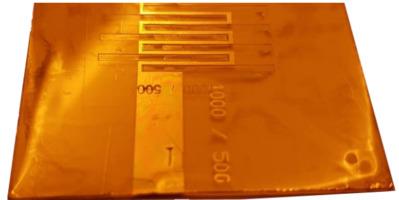
Fig. 5. Photograph of a completed micro-heater implemented on a thermoforming master. The micro-heater is matched between the trenches with big electrodes at both ends for easy electrical contacting.
