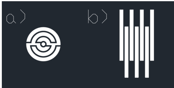
Fig. 3. Schematic of the thermoforming master for a) circular and b) parallel trenches.
