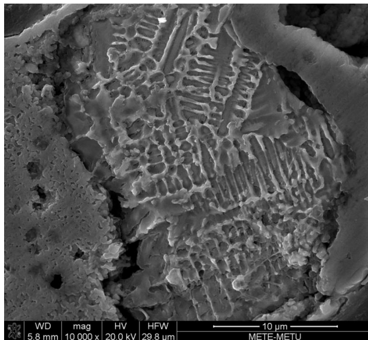
Figure 4.19 Dendritic microstructure of as-atomized powder particle
