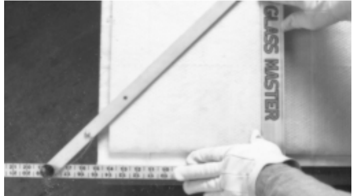
3. Place squaring tool on duct board so rule edge is parallel with factory female shiplap. Line up inside duct width dimension on rule with right hand edge of cut made in Step 2.
