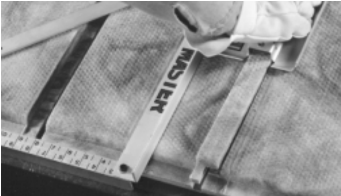
6. Rotate corner grooving tool end-for-end (or use next sequentially numbered tool) and place along guide edge of squaring tool to cut second corner groove. Remove groove scrap.
