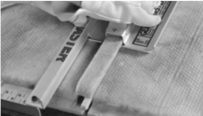
7. Re-position squaring tool to the right, to line up desired inside duct width dimension as in Step 3. Cut third corner groove using tool as in Step 4.
