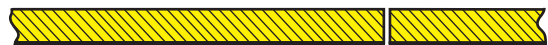
#SCO. Straight cutoff tool. May be used with #R1 to make the same cut as #7 tool.
