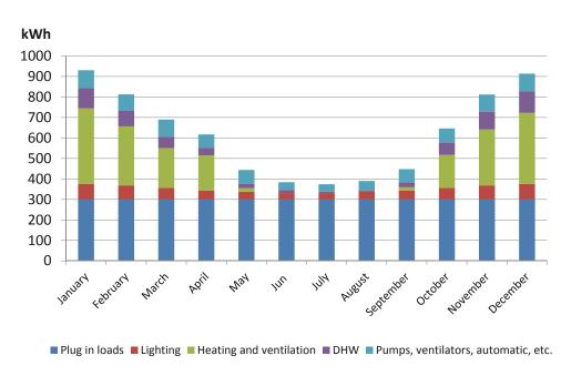
Figure 3. Break down of building electricity consumption by month.
