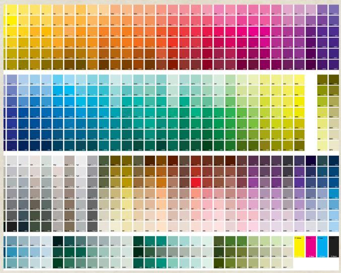
Every combination of ink and substrate has some limits in terms of colour gamut. Make sure you know if the colour you hope to achieve is within the gamut of the device that will be used, for example by having a colour sample printed using the exact same ink and substrate used for your project. This colour sample is provided by the English printing service Digetex.
