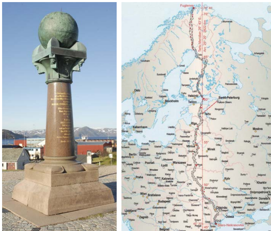
Figure 7. Left : the obelisk at Hammerfest is one of the geodetic points of measurement. The inscription reads 70^{\circ} 40' 12'' N, 23^{\circ} 39' 48'' E (photo CS). Right : Geodetic Arc map as displayed on site. Credit: National Land Survey of Finland.
