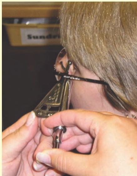
➔ Figure 1 The measurement of vertex distance using a vertex distance measuring gauge
