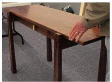
James Krenoff inspired this table design with the legs tapering up to the thin part of the taper at the top. The legs were coved on a tablesaw and thru wedged tenoned.
